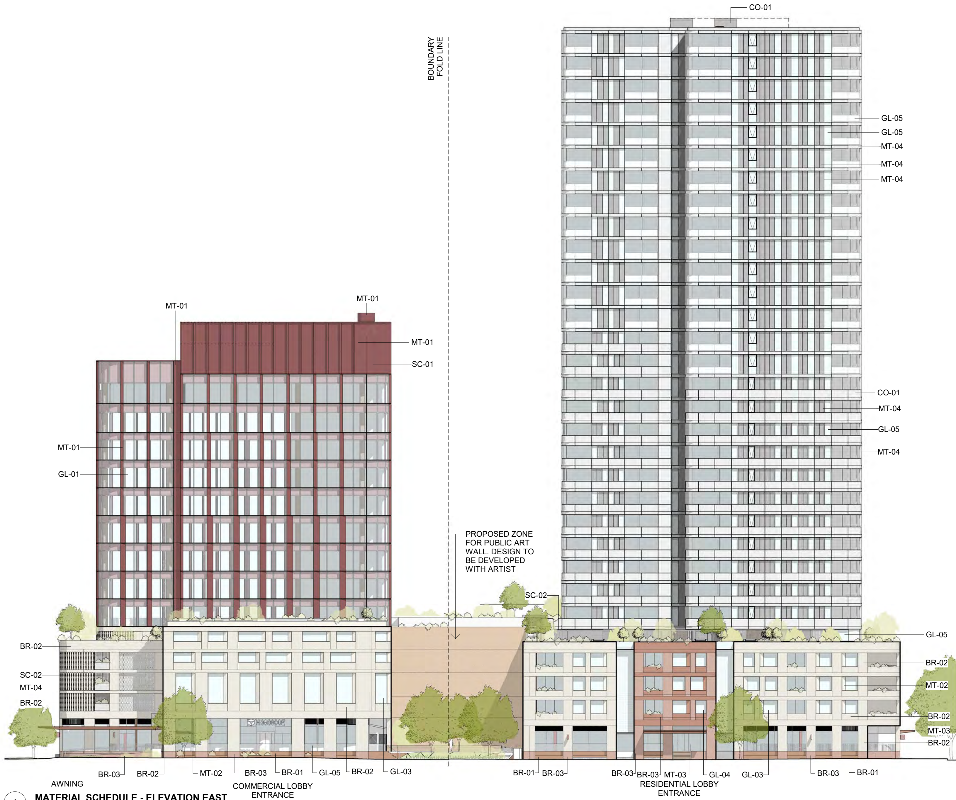
MT-01 - ALUMINIUM CLADDING (MANOR RED) ALUMINIUM CLADDING IN EARTHY OXIDE RED FINISH REF: DULUX MANOR RED
